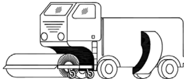
Pushed type sweeper special purpose vehicle integral engine/rear blower cab-over design small to large swath
