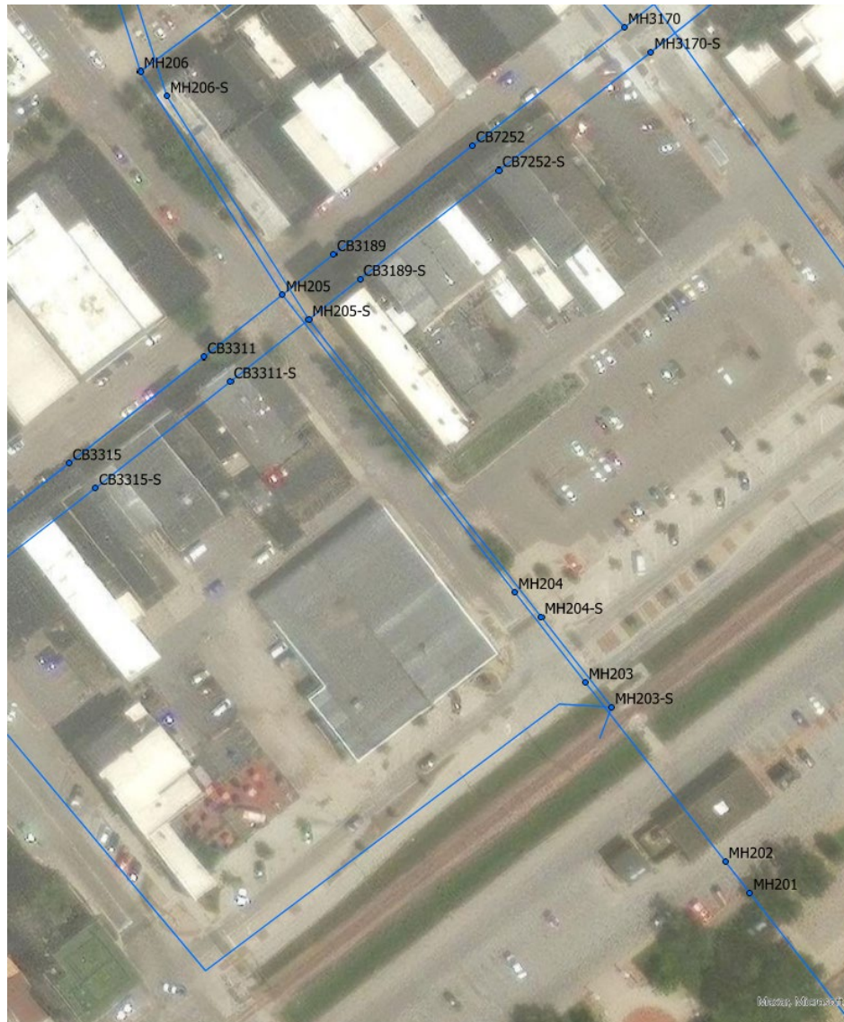
Figure 4-6: PC SWMM Links and Nodes
