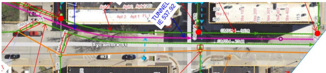
Figure 5-1: Rerouting of West Interceptor
