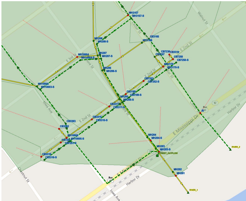
Figure 3-6: Flooding Junctions at Flood River Elevation
