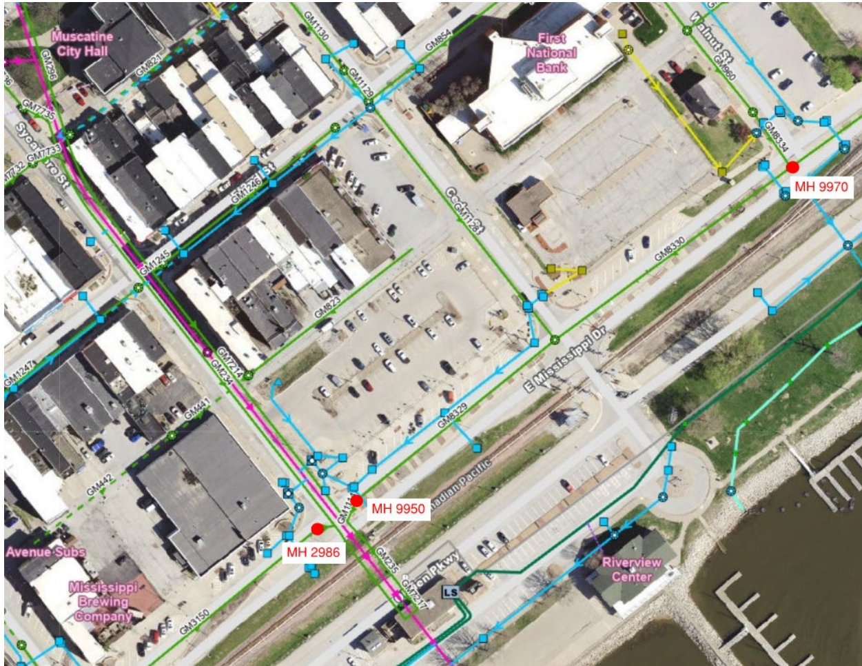
Figure 5-5: Manhole Surcharge Locations
