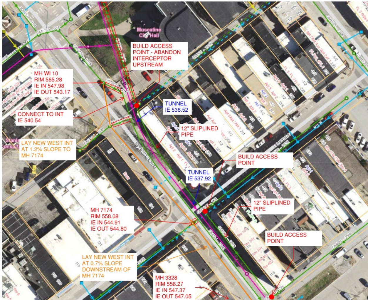
Figure 5-3: Rerouting of Sanitary Interceptors
